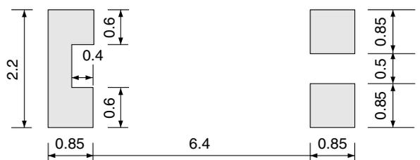
Note: Please make sure that there is no electric wire line under SSP-T6 on the circuit board.
